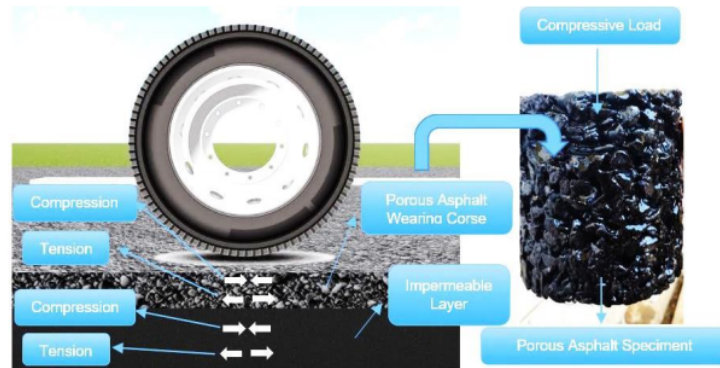
Figure 1. Surface layer including a layer made with porous asphalt when receiving vehicle loads
