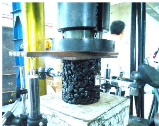
Figure 2. Equipment of compressive strength test
